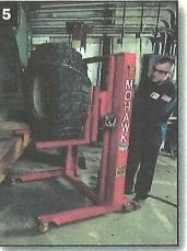
▲ Counterbalanced air-hydraulic tire dolly makes removing heavy truck tires a simple & safe one man job.
